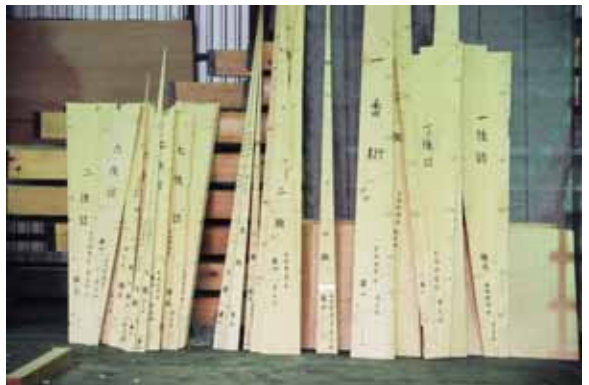
Photo 15: Templates Produced for Heisei Era Renovation
